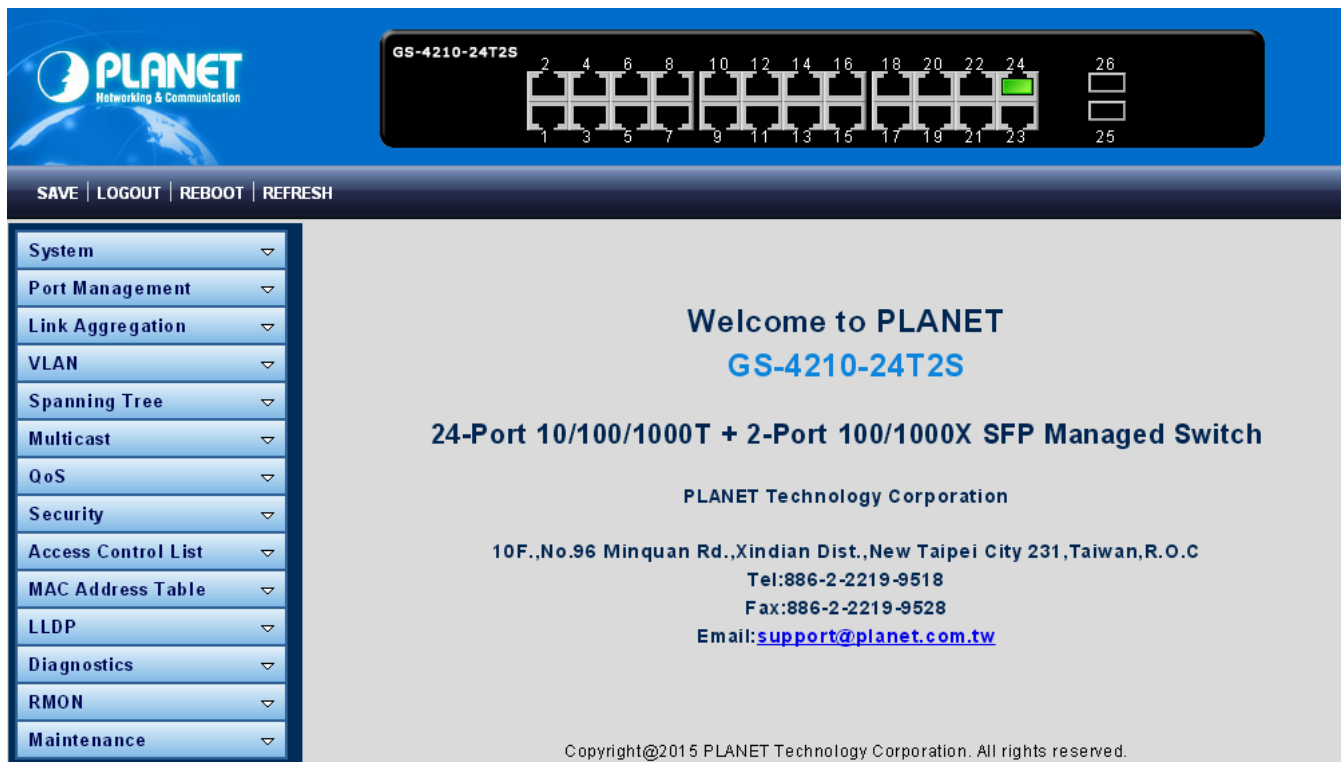
Figure 3-4: Web Main Screen of Managed Switch
