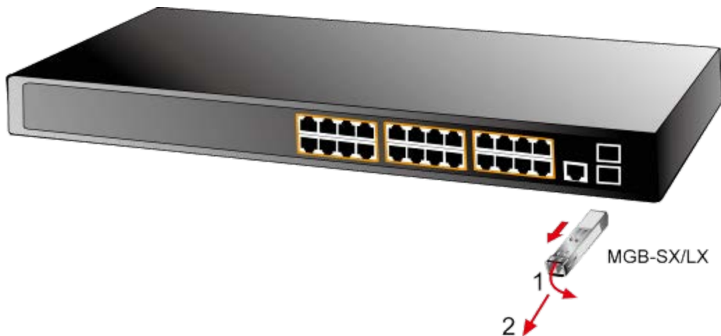
Figure 2-1-18: How to Pull Out the SFP Transceiver
